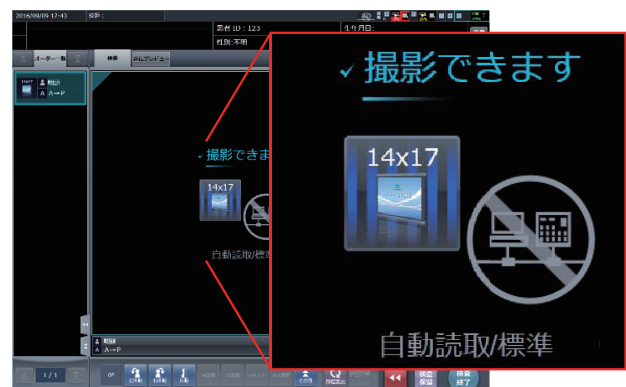
Fig. 7 Operation window for performing general radiography using Aero DR panel.
